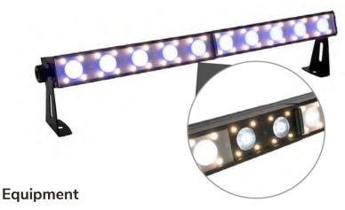
Two types of LEDs are used: Each segment consists of 5 powerful 15 Watt RGBW LEDs. The entire system therefore consists of 20 LEDs for the colored light. Each of these LEDs is individually controllable. The beam angle of the LEDs is 8 degrees, but you can widen it considerably using the frost filter supplied. The colored LEDs are optically complemented by a total of 80 warm white LEDs, which provide structure on the left and right and can be controlled separately for each segment.
