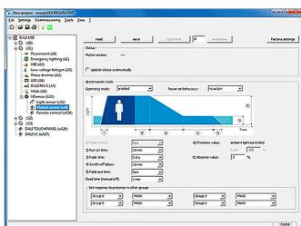
In addition, all the parameters of driver PRE can be configured for maximum effect. The current can be adjusted in 1 mA increments for individual matching to the required luminous fluxes.
