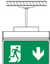
Ceiling mounting with extension rod 0,25-1m
