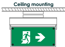
Recessed ceiling mounting on suspended ceiling with mounting base
