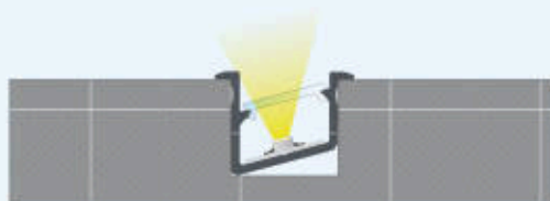
The effect of mounting V LED profile with BASIC cover in a milled hole.
