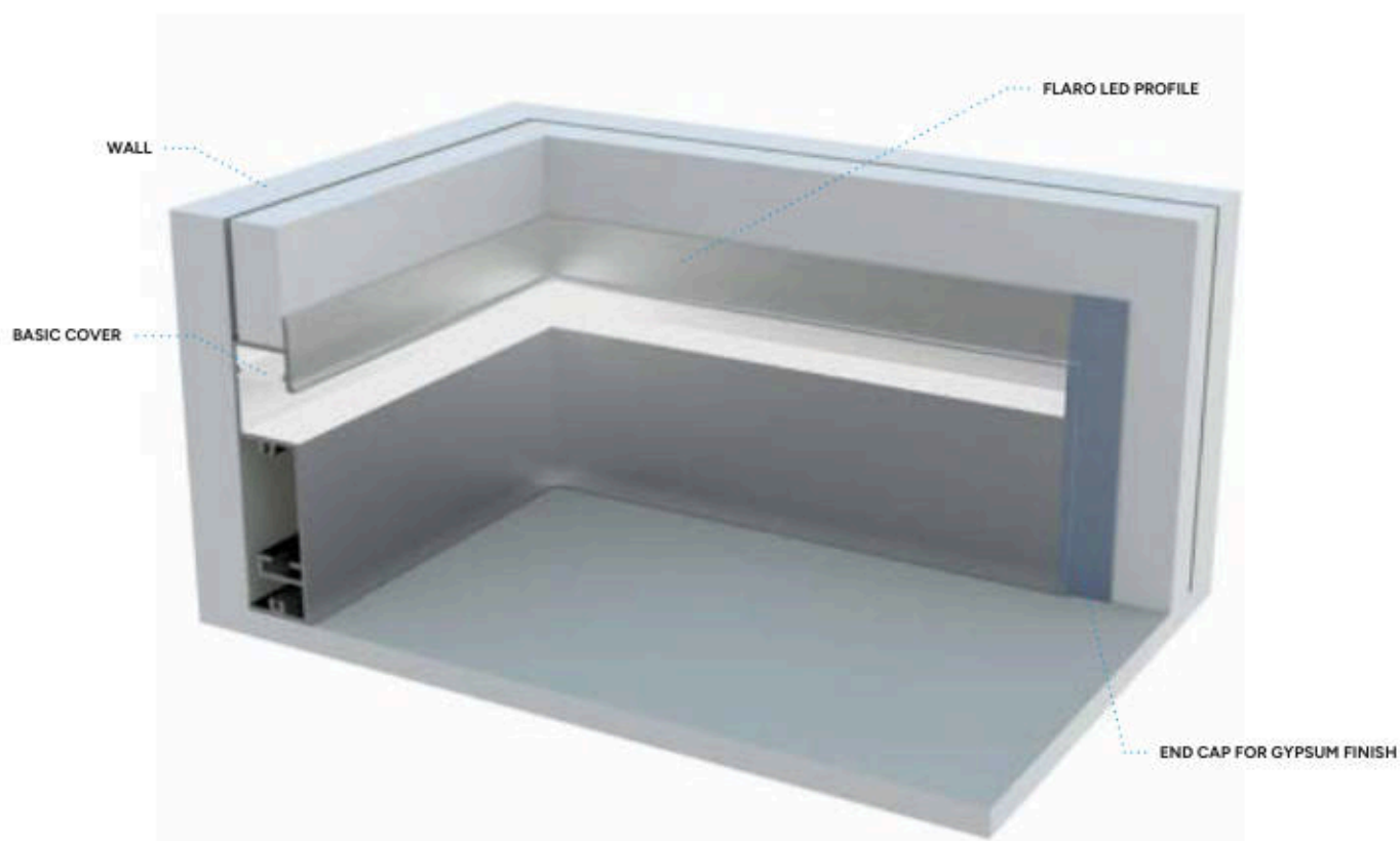
The effect of mounting two FLARO LED profiles with BASIC covers connected with 90° angular transverse connector .
