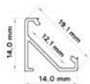
BARDE ALUMINIUM LED PROFILE 1 PC
