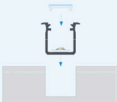
Instructions for installing G LED profile with BASIC cover in a milled hole.
