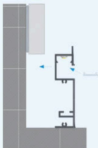
Instructions for installing FLARO LED profile with BASIC cover .
