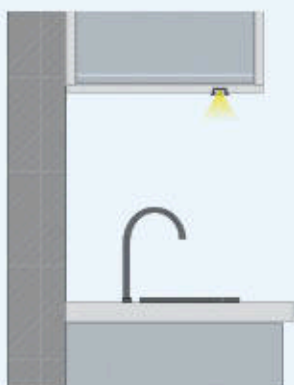
Example of installing Z LED profile in a milled hole in a cabinet above the kitchen countertop.
