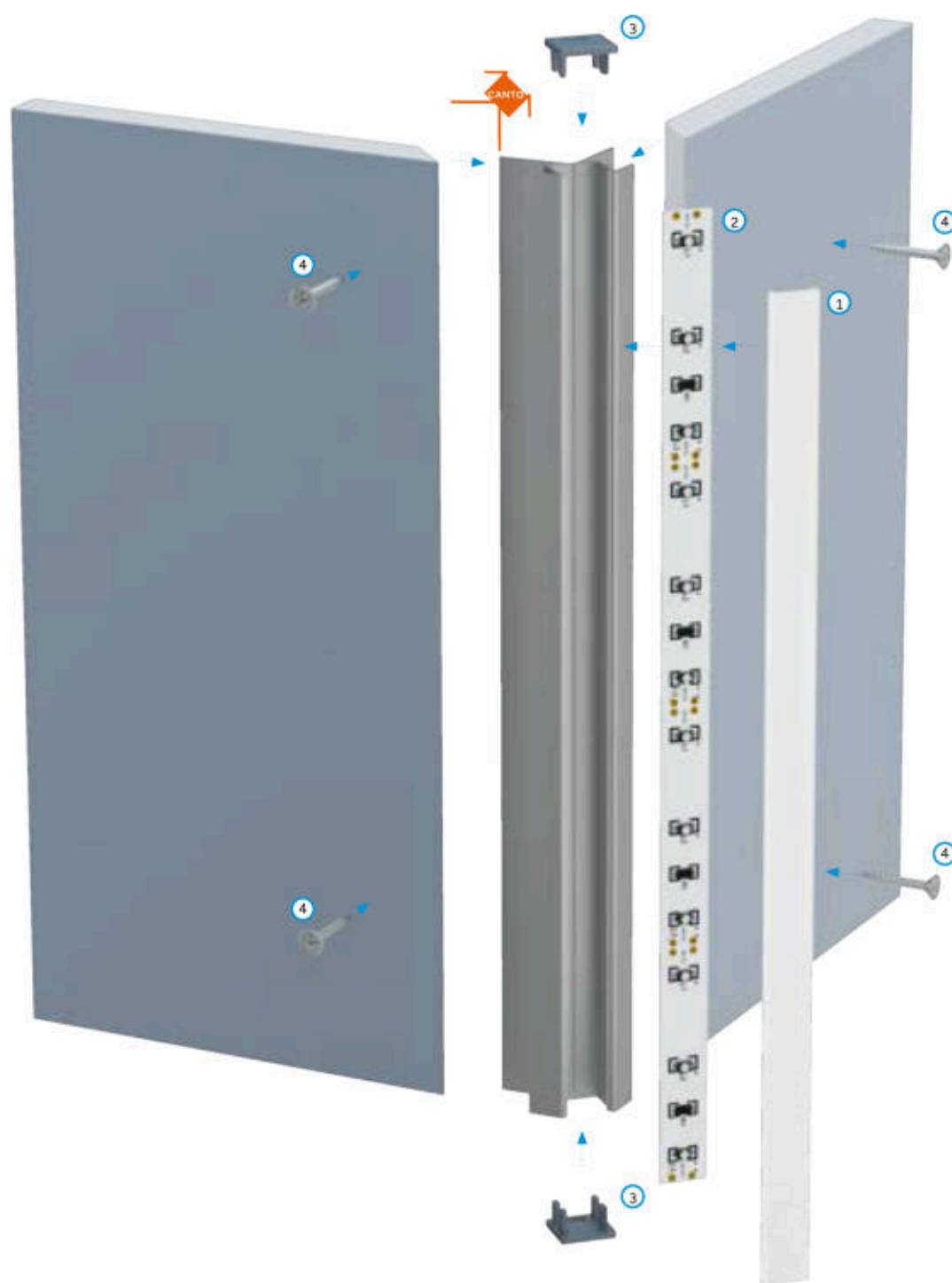
Assembly scheme for elements of the lighting system using CANTO non-perforated LED profile and (1) BASIC cover , (2) LED strip , (3) end caps with holes , (4) screws .
