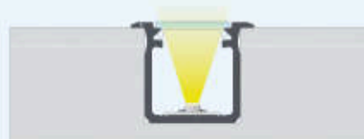
The effect of mounting G LED profile with BASIC cover in a milled hole.
