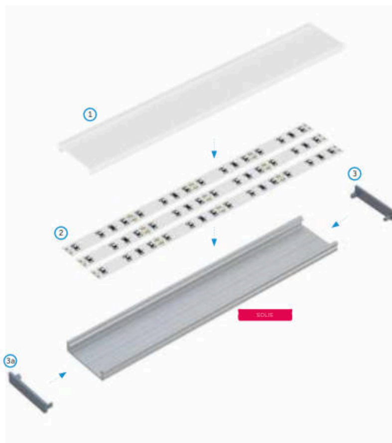
Assembly scheme for elements of the lighting system using SOLIS LED profile and (1) WIDE cover , (2) three LED strips , (3) end cap without hole , (3a) end cap with hole .
