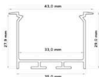
HEDE ALUMINIUM LED PROFILE 1 PC
